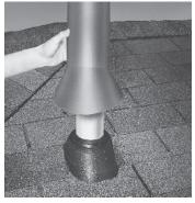
Place CapMaster over pipe and rotate to proper angle. Friction clips hold it in place.
