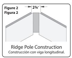
better if it extends the entire length of the roof and therefore blends in with the roof line. Measure the length of the roof peak to determine the total length of OmniRidge® Pro Vent one will need. NOTE: DO NOT CUT THE HOLE THE ENTIRE LENGTH OF THE RIDGE. THE LENGTH OF THE CUT WILL BE ONE (1) FOOT LESS THAN THE LENGTH BETWEEN THE END WALLS (SEE STEP 3).
