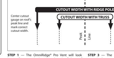
Center cutout **CUTOUT WIDTH WITH TRUSS** gauge on roof's peak line and mark correct cutout width. **STEP 3** — The width of the cut will depend
