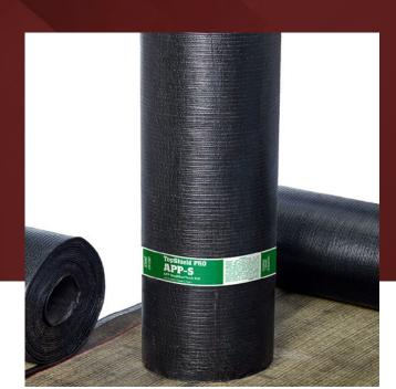
Product Composition and Features: TopShield® PRO modified bitumen membranes are manufactured on state-of-the-art, dedicated roofing lines that were exclusively designed for the production of modified bitumen products. TopShield® PRO APP-S is produced with a high performance, stress-resistant polyester mat that is impregnated and coated with a superior grade, modified bitumen compound.
